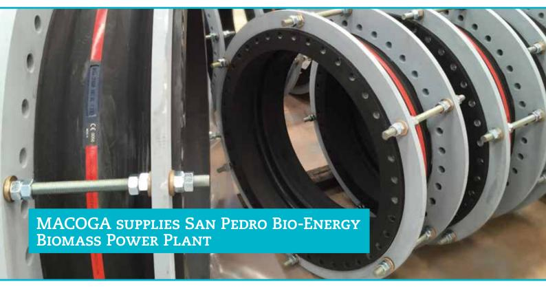
MACOGA has successfully manufactured a large number of metallic and rubber expansion joints for the San Pedro Bio-Energy Biomass Power Plant.
